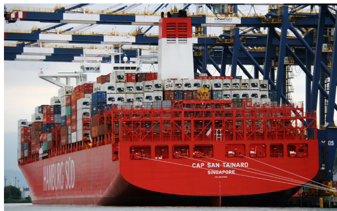
Hamburg Süd's 9,600 teu Cap San class vessels are among the world's largest reefer ships.
