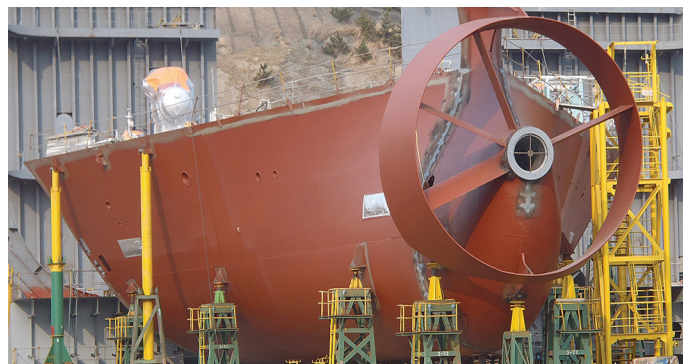
Installing a Mewis Duct and a more suitable rudder will give a payback on a five-year-old VLCC in a few months, says UBS.
